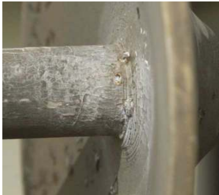
Figure 7: The visible damage of punctures along the sheath of the test insulator
