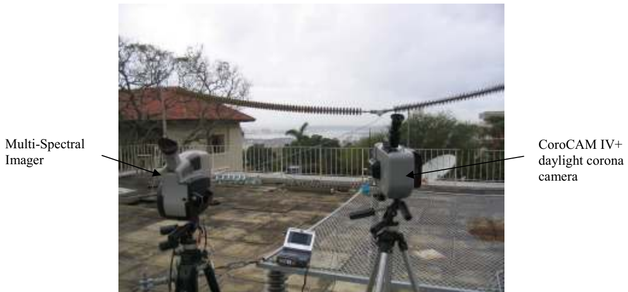
Figure 6 The Kwazulu Natal University test set up, on the left the Multi-spectral Imager, on the right the CoroCAM IV+ corona camera and in the background the suspended non ceramic insulator.
