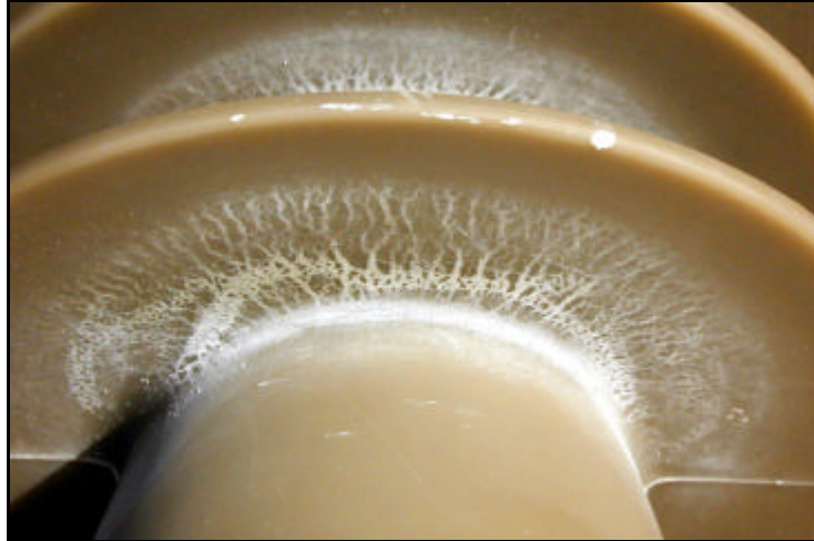
Figure 5: Effects of 9 Hour Mould Release Resiliency Test (Leakage Current) on CE insulator Surface.
