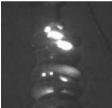
Figure 7 : Onset of discharge activity at dead end after ~30 minutes stressing. V=173 kV rms.
