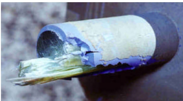
Fig.4.2-1 : Brittle fracture about 1 cm inside the end fitting.
