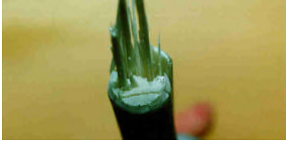
Fig. 4-1 : Failure pattern of a brittle fracture
